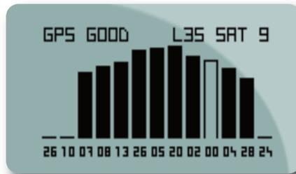
Please note: for a quick GPS signal acquisition place Solo in the open air so that a wide part of the sky is visible.
